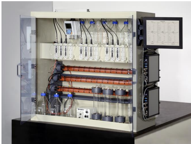
Column test facility – for the leaching of ores and minerals
